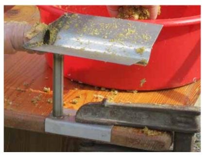
Picture 3-6: Funnel used to stuff chamomile, fixed on the table using a clamp
